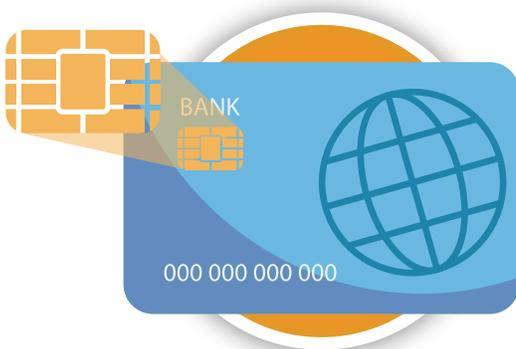
A chip card has an embedded microprocessor chip (it looks like a small, metallic square on the front of the card) that stores information securely and performs cryptographic processing during the payment transaction.
